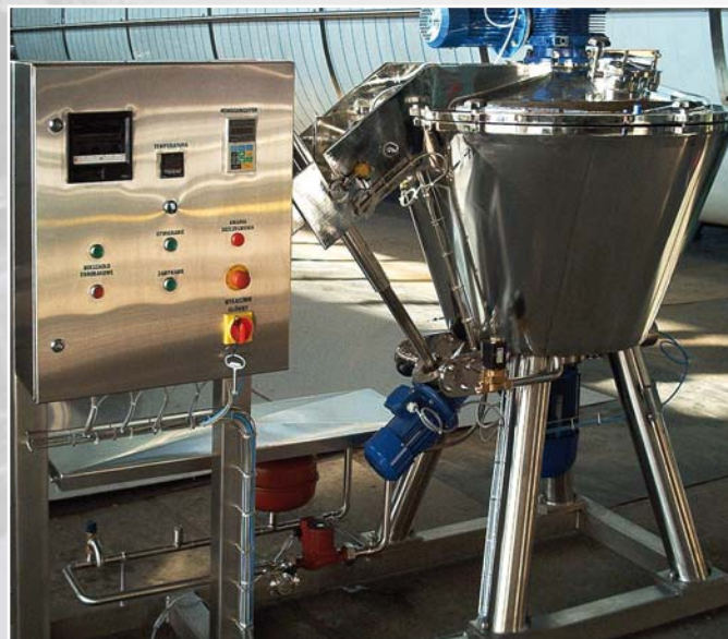
A conical mixer with a homogenizing agitator and a gate agitator, equipped with an electric heating system
