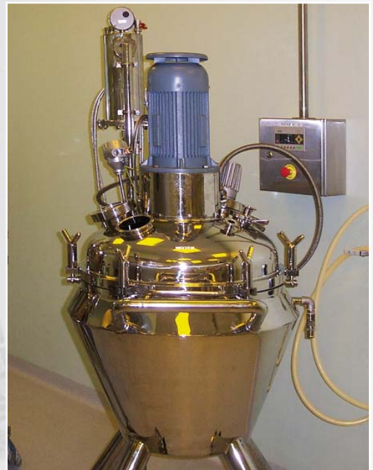
A conical mixer with a propeller agitator (made to Ex zone standards)
