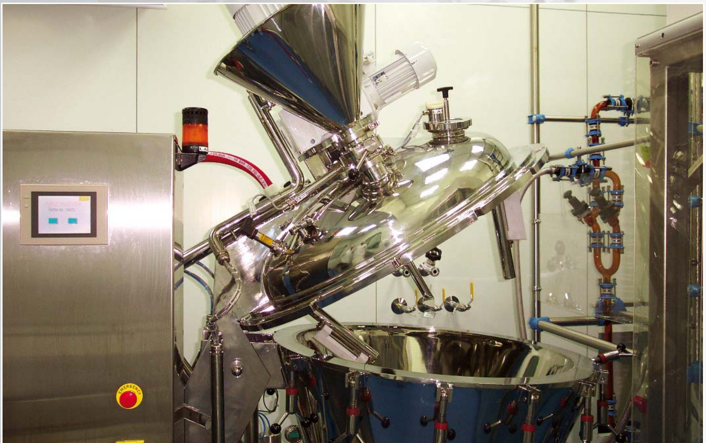
An open lid of a conical mixer with a gate and paddle agitator
