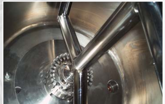
A homogenizing agitator at the bottom of a vessel and a gate agitator
