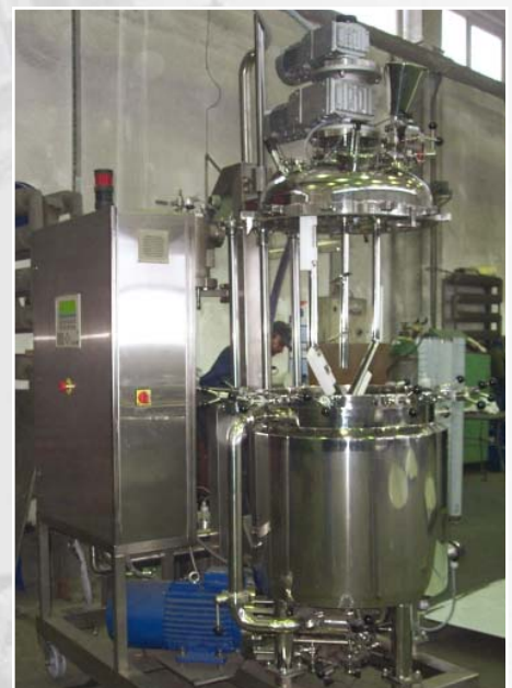
A laboratory homogenizing mixer, V=100 L
