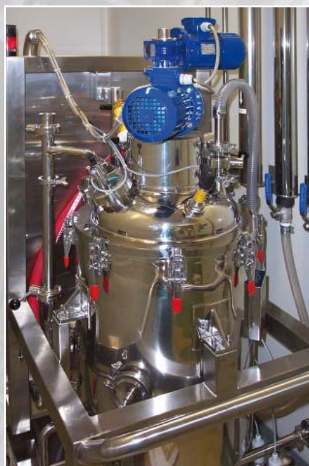
A laboratory homogenizing mixer, V=50 L
