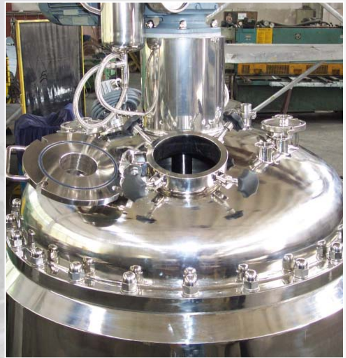
A reactor adapted to operate in a potentially explosive atmosphere
