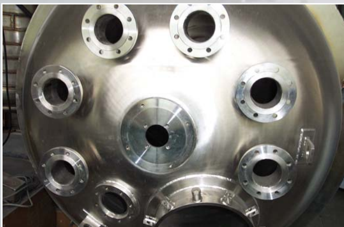
A pressure vessel head with stub pipes
