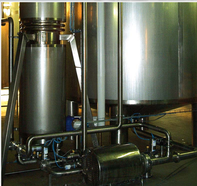
A shell-and-tube heat exchanger with heat compensation
